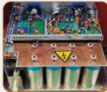
500 kVA recovery energy inverter, prototype
