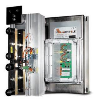
ME-VLD-A makes negative to earth connection using anti-parallel connected thyristors; they are controlled by a dedicated trigger board and control unit.
